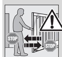
All persons using the gate system must be shown how to operate it properly and safely. Demonstrate and test the mechanical release as well as the safety return. To do this, halt the closing gate by grasping it with both hands. The gate system must initiate the safety return.
